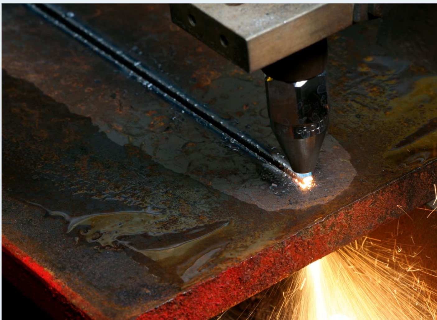
Water puddles formed on a cool plate during oxy-propane cutting. Moisture leads to corrosion and causes problems when preheating, brazing or welding.
